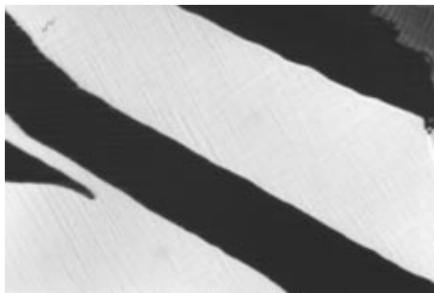
Fig. 10 A representative POM image of an as-synthesized mesoporous silica film on mica (image size is 150 × 120 \mu\text{m} )
